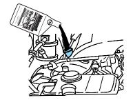
• Do not overfill the engine with oil. Oil levels above this mark may cause engine damage. If the engine is overfilled, some oil must be
